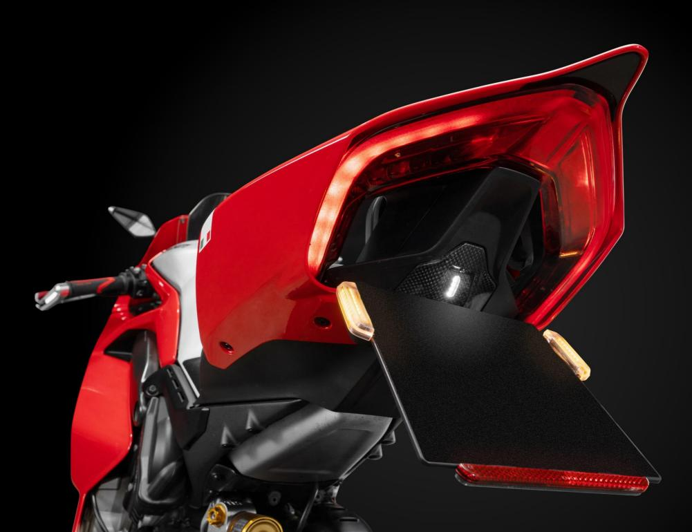
Carbon fiber attachment with integrated LED license plate light, available in matt or glossy fiber carbon . Perfect interchangeability with the original holder.
